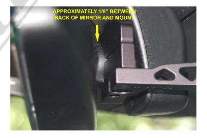
STEP 2 - Tighten the clamp screw until the Top and Mid Sections are slightly snug around the mirror stem. You should still be able to move the mount along the stem. Before fully tightening the clamp screw, slide the mount towards the windshield as far as it will go. There should be approximately 1/8" between the back of the mirror and the mount as shown above.
