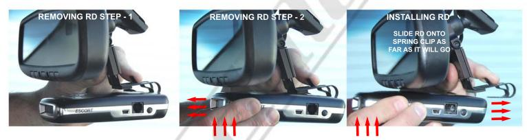
VERY IMPORTANT - When removing or installing the RD, squeeze the trigger and the back side of the mount together with one hand, and lift the front of the RD upward with the other hand before sliding the RD off or onto the spring clip. You must lift the front of the RD upward before sliding it off or onto the mount.
