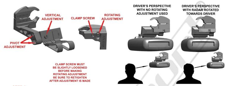
**STEP 3** - Install your radar detector onto the mount. Use the adjustments shown above to adjust the RD to your desired position. We recommend adjusting the RD as close to the bottom of your mirror as you can. **NOTE** When the rotating adjustment is used to rotate the RD towards the driver, the footprint of the RD is reduced as shown above. Be sure to tighten all of the adjustment screws after the adjustments are made.
